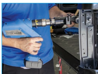
Use the Blind Rivet Adapter with the Henrob Conversion Kit
