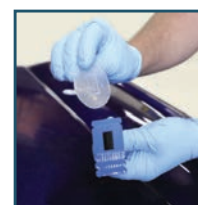
Plastic tabs are reusable and ready to pull dent after dent.
