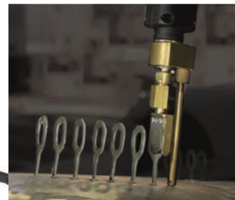
Apply keys and studs with Drawn Arc Welding
