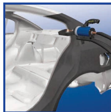
Spot welding a quarter panel using C-Arm (PS-302).
