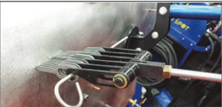
PULL BAR DENT PULLING
