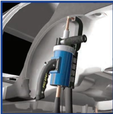
Wheelhouse arm applies consistent welds in difficult areas like the wheelhouse.
