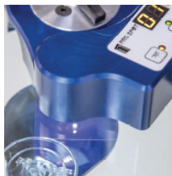
Step 3: Use the tool's UV light function to cure the resin
